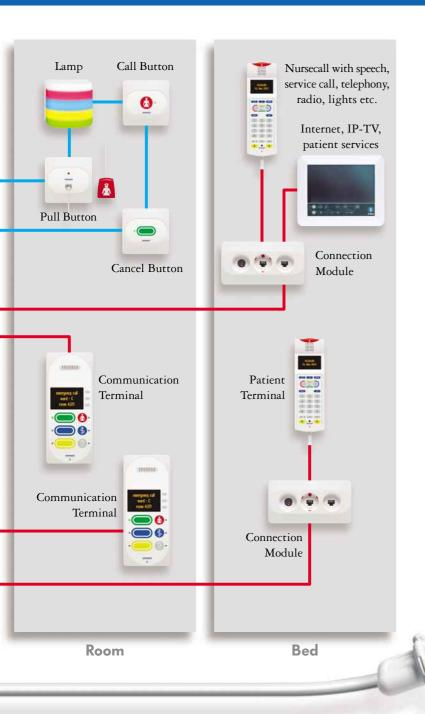
For the increasingly more complicated communications needs in hospitals, VISOCALL IP is taking a decisive step forward. As an autonomous nursecall system in a multimedia-capable communications platform VISOCALL IP combines many functions in a single system.
